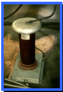
Marca: HIPOTRONICS Part No: BFR-1599-A314 Capacitance: .001 \mu F Voltage: 100KV Frecuency: 50/60Hz
