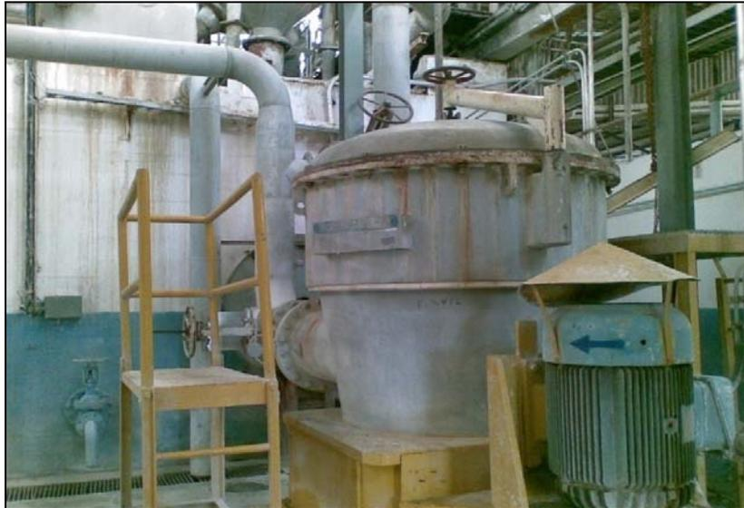
Figura 3.10 Depurador vertical primario (Fine screen N°1).
