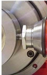
**Figura 2.4.** Ensayo Pin- On- Ring. (Tribology-ABC, 2010)
